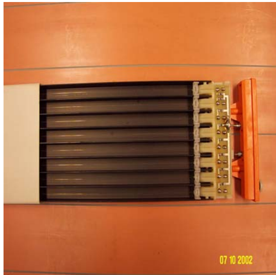
Figure 1. Photo of a standard LST, partially inserted in the sleeves (shown on the left).
