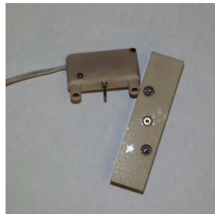
Figure 19. Opened prototype HV connector (left), connector plus endcap (right).
